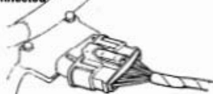
Connector disconnected or improperly connected
